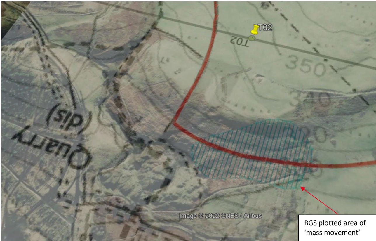
Figure 10: NE Oblique View Showing Mass Movement including BGS Mapped Areas
