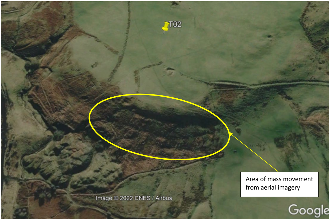
Figure 9: NE Oblique View showing Mass Movement
